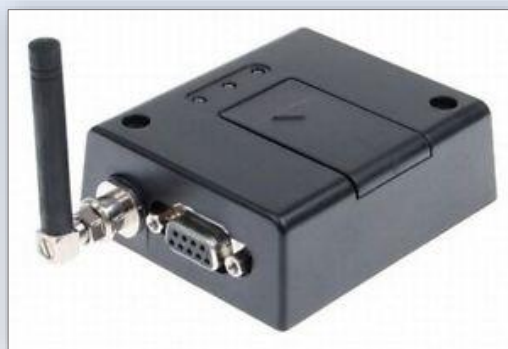
Left: detail of a DISPLAYCE receiver, configurable as "node" or "gateway". Right: detail of a UMTS modem that can be interfaced with the gateway.
